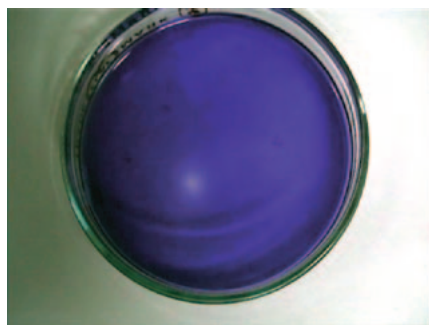
Fig. 3. Color change of aqueous phase with m -Cresol Purple. The elapsed time after contact between the organic and aqueous phases is 3.5 s. The most distinct colorless portion exhibits the pH being almost neutral. Purple portion corresponds to pH \approx 11. The colorless portion appears randomly anywhere in the interface and fades out gradually. Concentrations of \text{Ca}(\text{OH})_2 and DEHPA are 1 and 5 mM, respectively.
